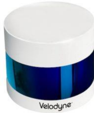
Figure 4: A Velodyne Puck 32MR. Lidar device. Source: Velodyne
