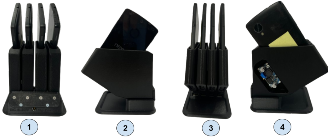
Figure 4.5: Cloudlet 3D rack prototype. (1) the back side, (2) the left side, (3) the front side, and (4) the right side.
