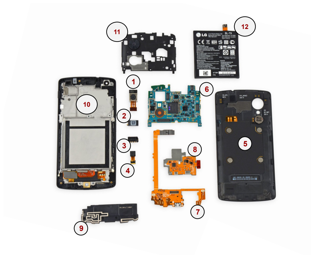
Figure 3.9: Nexus 5 phone components disassembled with each number representing: 1. 8MP rear-facing camera, 2. Earpiece speaker, 3. Headphone jack, 4. 1.3MP front-facing camera, 5. Back case, 6. Motherboard, 7. Daughterboard, 8. LG D821 Nexus 5 Flex Platine PCB Assembly Sub, 9. Speaker, 10. Display, 11. Motherboard cover, 12. Battery.
