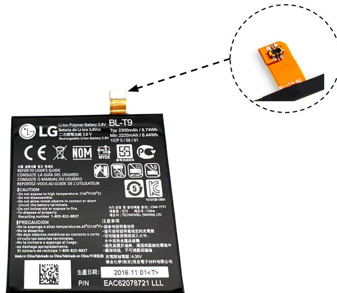
Figure 3.4: Google Nexus 5 battery BL-t9 2300 mAh.
