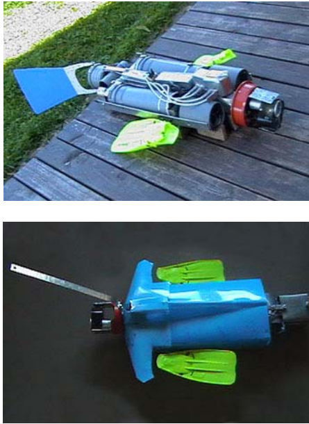
Fig 1. Second prototype without protective cover and with towing rod attached.
