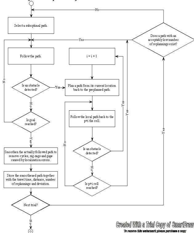
Fig. 16. Path selection algorithm with local replanning
