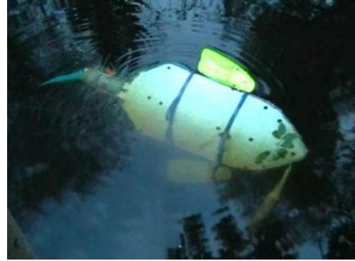
Fig. 6. Pond test. Robot surfaces in vertical mode using only one side balloon.
